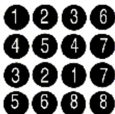
Figure 10: The 4x4 duplication pattern used in the production of the filter sample3-4x4b .
